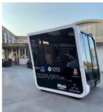
Figure 2: The NEXT system: modular pod for passengers and cargo hitching
